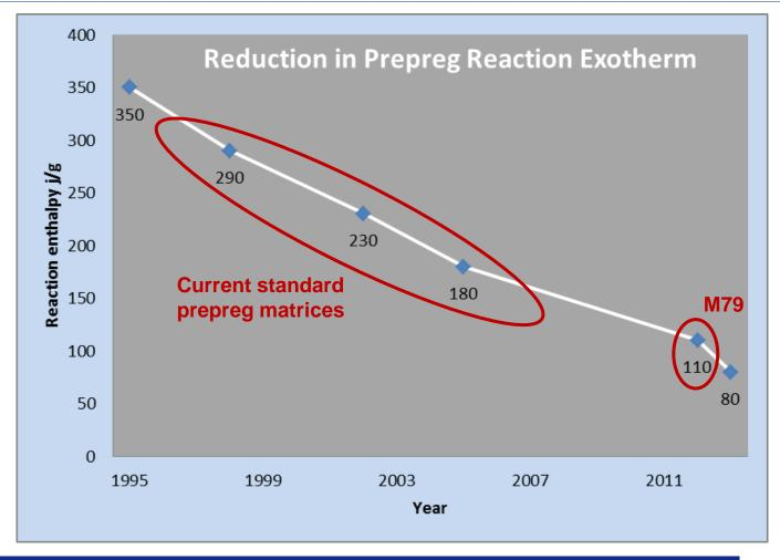
Latest prepreg matrices minimise reaction exotherm allowing short cure cycles of thick structures
