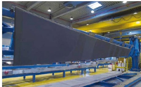
A350 XWB wing spar prototype manufactured by GKN using HexPly® prepreg
